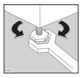
Any necessary adjustment can be made with a spanner. Accurate levelling prevents vibration, noise and displacement of the machine during operation. Some vibration is inevitable, especially if mounted on a wooden floor.
